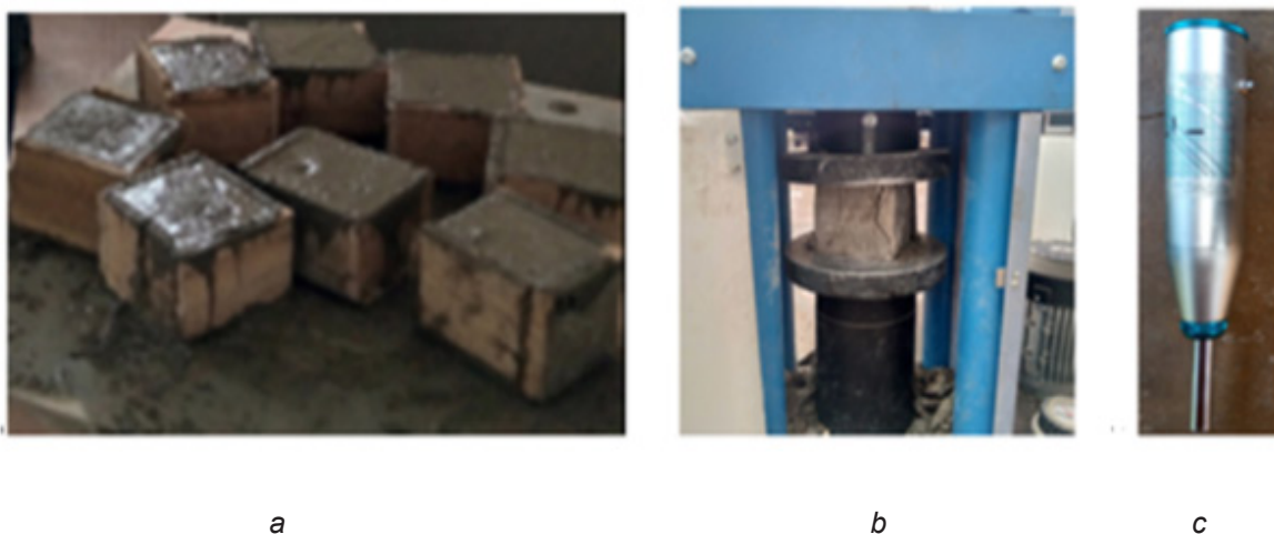
Figure 1 – Experimental samples preparation (a) and compression testing under hydraulic press (b) and sclerometer (c) used in the laboratory and in-situ study Source: compiled by the authors.
